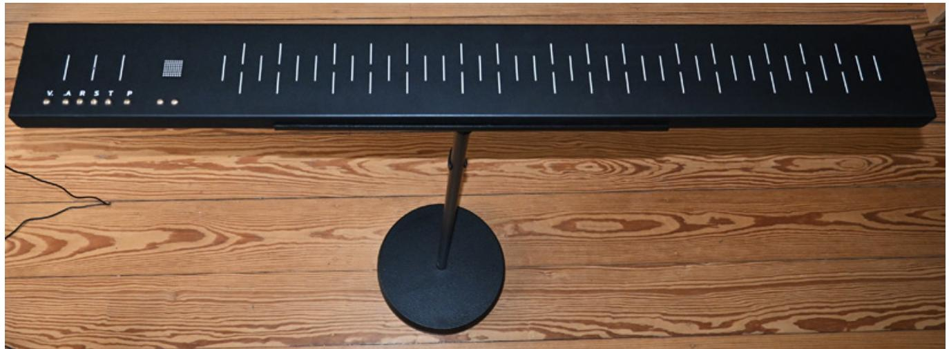
We tested it as described on the König & Meyer 26000 tripod with a large, heavy cast base (see fig. above). This works well - even during operation - as the capacitive buttons do not exert any significant mechanical pressure on the Flux. Lighter tripods can also be used for mobile applications, such as the 19900 from König & Meyer.
