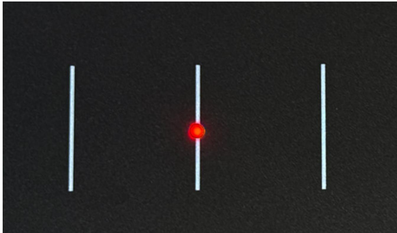
The modulation field is located on the left. Depending on the selected algorithm, there is either a large area over which the magnet can be moved in all three dimensions to produce modulation, or the modulation range is divided into three lines, which are also marked with white lines on the field. In this case, three parameters can be adjusted in two dimensions (position and distance). Actually, it sounds more complicated than it actually is.
