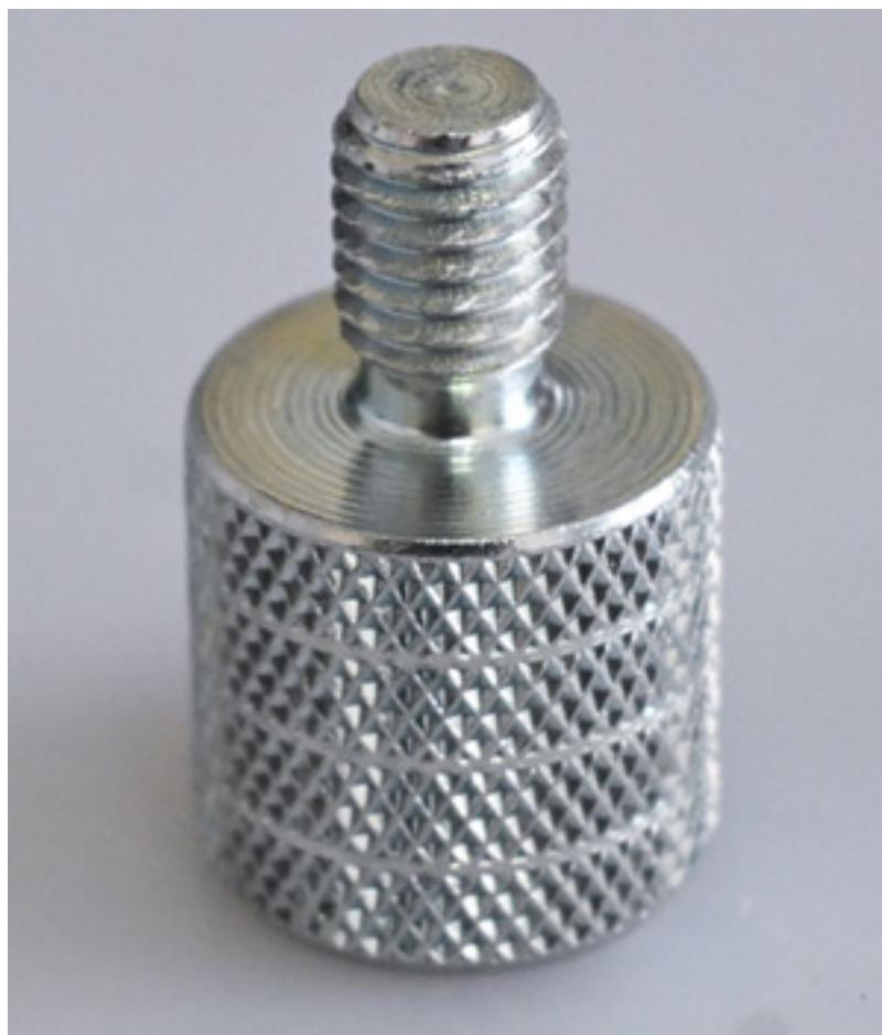
With the 21918 adapter from König & Meyer (see image above), the Flux Speaker Stand Adapter can also be attached to a microphone stand with a 3/8-inch threaded screw. The M8 screw thread (see image above) is 30mm long and, as the screw protrudes into the adapter and hits the Flux, you will need to use a few washers from a hardware store, place them on the adapter, and also obtain an M8 nut for fastening.
