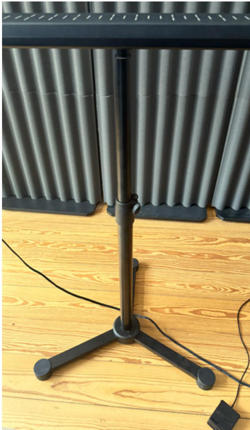
However, it is simpler and more stable to use a robust speaker stand with an 8mm screw, such as the König & Meyer 26720. No DIY work is required - and everything fits perfectly. The better fastening and thicker tube make the whole setup much more stable, making it highly recommended for studio use.
