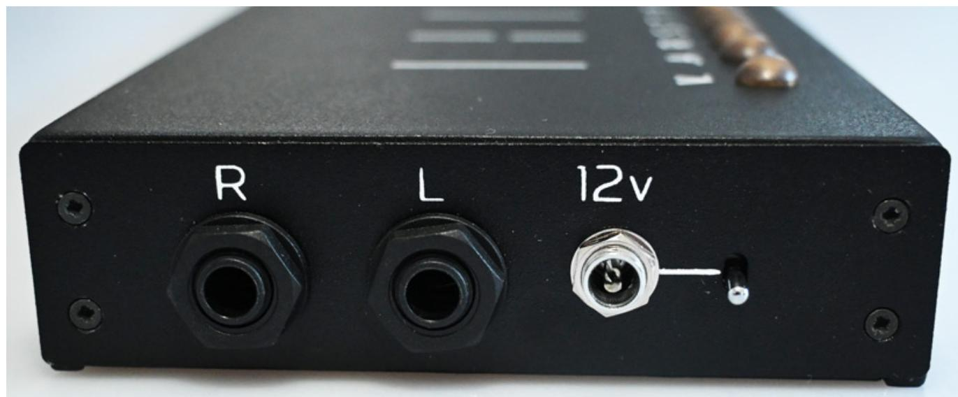
The connections for the Flux are located on both sides. On the left side are the two 6.3mm jack sockets for the audio outputs (18 V pp) and the socket (for 2.1mm hollow plugs with positive pole in the middle) for the supplied power supply unit with a 12-volt operating voltage (0.4 ampere operating current). Next to the socket is the switch for turning the Flux on and off.
