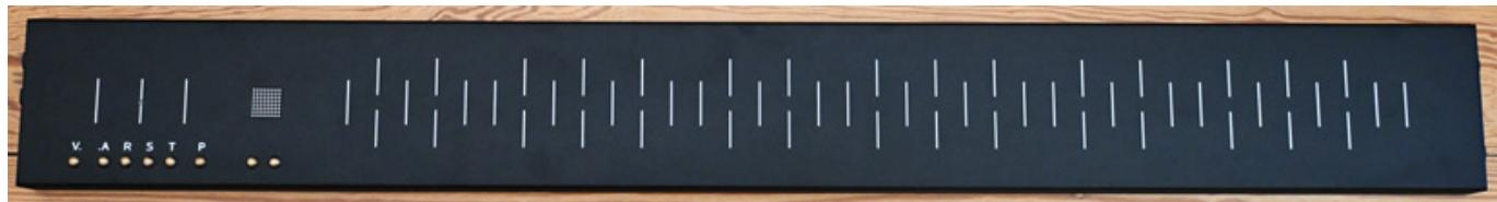
There are two areas on the Flux surface: on the right is the area for triggering the tones and controlling the pitch and volume, and on the left is the area for the various modulation options.
