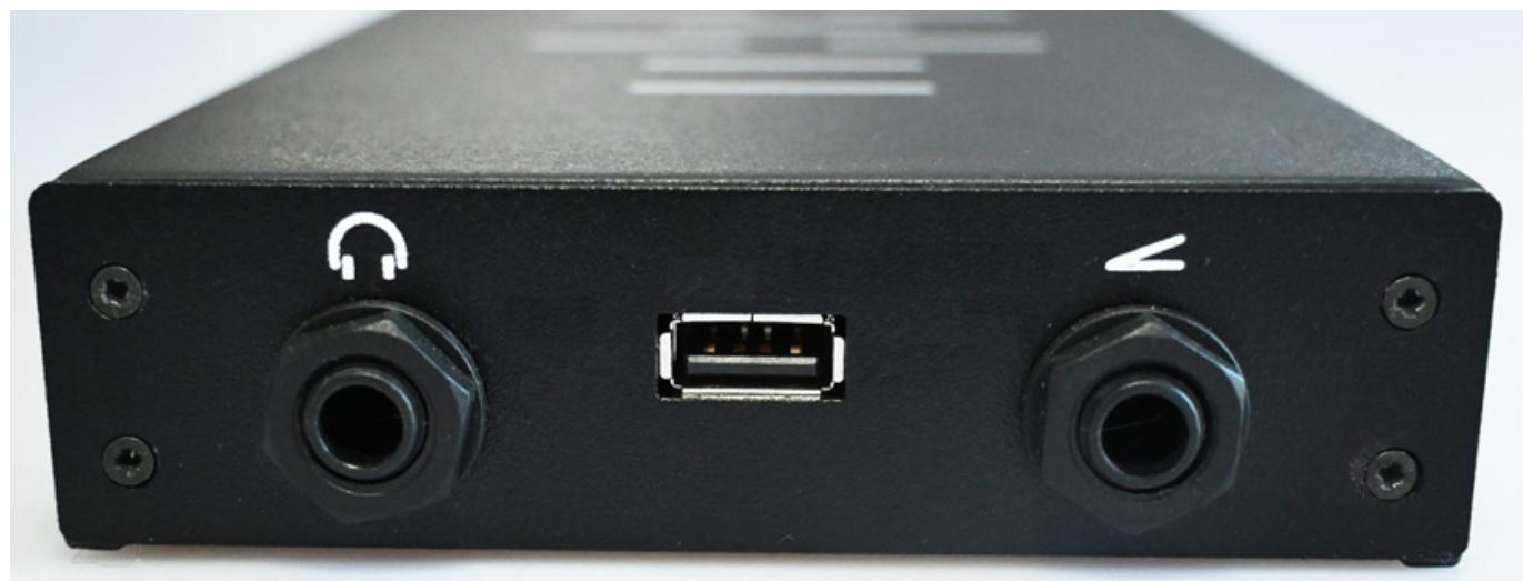
On the other side is a stereo headphone output to which headphones with an impedance of 6 to 64 ohms can be connected. A foot switch can also be connected via another 6.3mm jack socket. The switch polarity is automatically detected when the device is switched on. There is also a USB-A socket for connecting a USB stick to transfer presets and update the Flux firmware.
