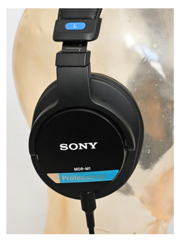
Like the MDR-MV1, the MDR-M1 is equipped with a 40mm dynamic driver. Visually, it looks very similar to the MDR-MV1, but the impedance is 50ohms, which is about twice as high as the acoustically open model. In addition, the installation and arrangement have also been slightly changed.
