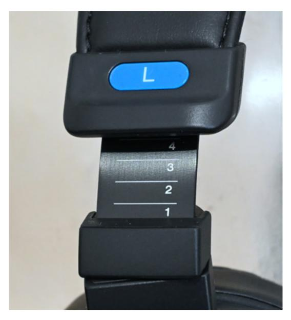
The headband can be adjusted by 40mm on each side in ten steps. It's nice that the individual adjustment points are marked and numbered (see image above) so that you can quickly set the same adjustment on both sides.
