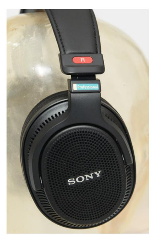
The headband can be extended up to 40mm on each side. This is enough for even large heads. A scale is embossed on the inner headband so that you can quickly find your desired setting, and the left and right sides are also marked with letters and the colors red and blue. The headphones weigh 223 grams without the cable.
