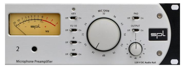
The SPL Crescendo Duo offers two input channels with up to 70dB of gain and two outputs per channel, the gain of which can be boosted by 10dB using the "Output"-switch independently of the input gain. This allows the user to feed optimal signal level to components further down the chain. The large rotary knob is detented, internally raising the gain by increasing amounts from +1 over +4 up to +7dB. The rotary control for output gain is stepless.
