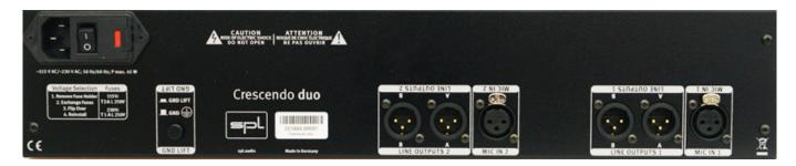
The rear of the enclosure sports an IEC socket, on/off-switch, one XLR input per channel plus two parallel line-level XLR outputs. Very useful for backup purposes. Input impedance is rated at ten kiloohm and output-impedance at 75 ohm. The maximal output level goes up to 32.5dBu. The phantom-power circuit suplies a whopping 35mA per channel, satisfying even the most picky contenders.
