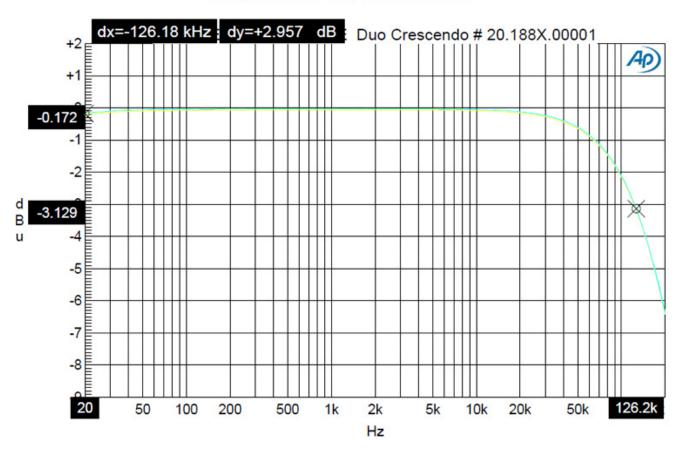
I have rarely seen such linearity in amplification over all frequencies from 20Hz up to 60kHz, with only a minute drop under 1dB!
