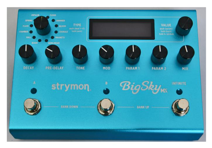
The functionality of the three foot-buttons has also changed. The first two on the left and in the middle are for the direct selection of one of two presets in a "bank" and the first on the far right is now for triggering the INFINITE function. This can be selected via the menu to a momentary function (Momentary) or an on/off switching function (Latching). By pressing the left/center or center/right buttons, the user can change the currently active bank (back or forward).
