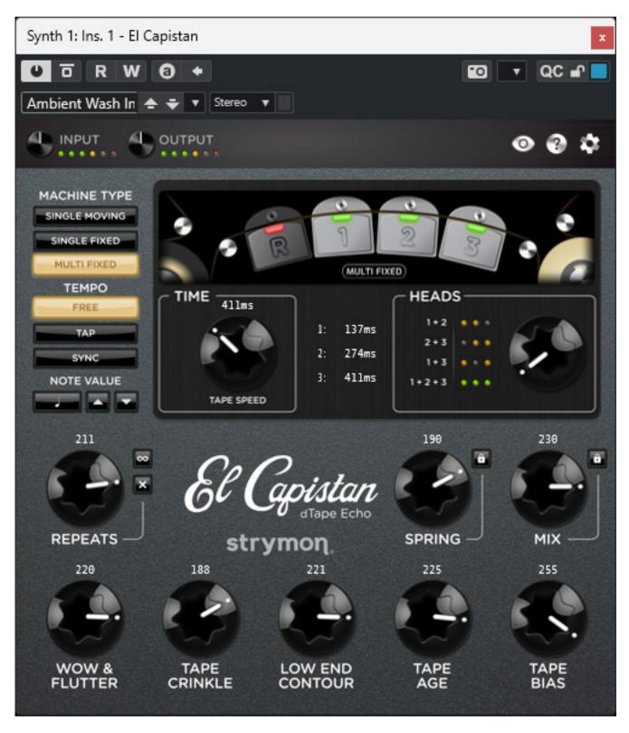
The El Capistan simulates an echo effect based on a tape loop with one recording and up to three playback heads, as known from the Roland Space Echo and the Watkins Copicat, for example. There are three different modes of arranging the two heads.
