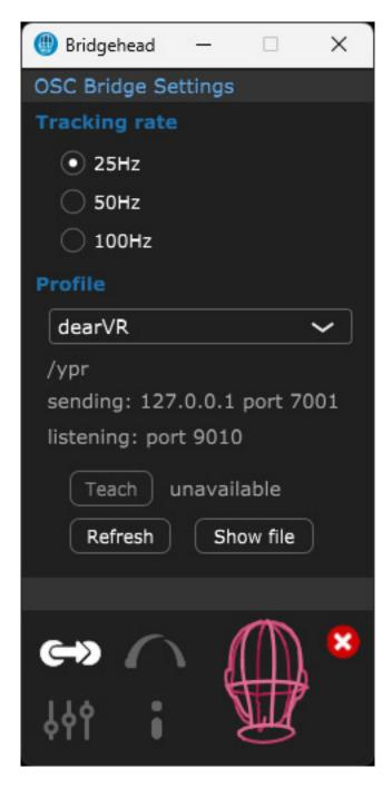
Communication between the head tracker and binauralizer plug-in takes place via the bridgehead using the OSC protocol. The position update data rate can also be set. In our experience, 25Hz is sufficient, and higher update rates may be too much for some DAWs.
