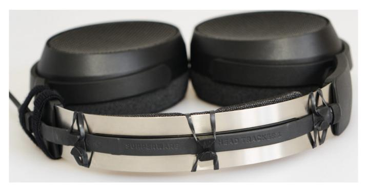
Using the Sennheiser HD 490 PRO as an example, we have shown how the head tracker band and USB cable can be attached using the rubber bands and clips provided and the two Velcro straps.
