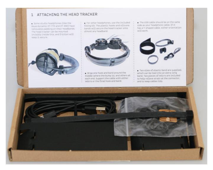
But now let's get to the product. The Head Tracker 1 is supplied with a quick start guide, USB cable, and fastening material in the form of eight elastic bands in two sizes with four plastic clips for the elastic bands for the head tracker band fastening and two Velcro straps for cable fastening.
