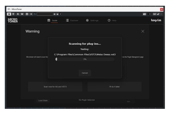
MicroToner is a plug-in that is integrated as a virtual instrument in the corresponding MIDI track via the VST instrument selection. After the first call, you have to scan the available virtual instruments (see figure above). Now you can call up the desired VST instrument within the plug-in and then make the corresponding settings in MicroToner concerning the scale.
