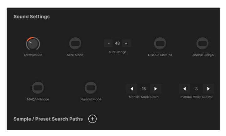
Here, you can deactivate effects, activate the MPE mode, and set the MPE range. The "MAQAM Mode" is used to activate compatibility with the MAQAM Quarter Tone Tuning Controller from Mazeka Toys. But that's something special for users from the Arab world. The Mandal Mode can be used to switch the microtuning per note. The switch is made with the keys in the specified octave.
