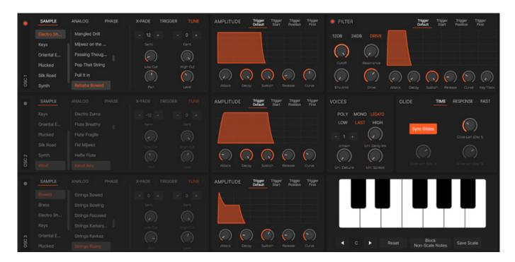
The synthesizer offers three oscillators. Behind each is a virtual VCA with an envelope generator, and the sum then goes to a filter with its own envelope generator.
