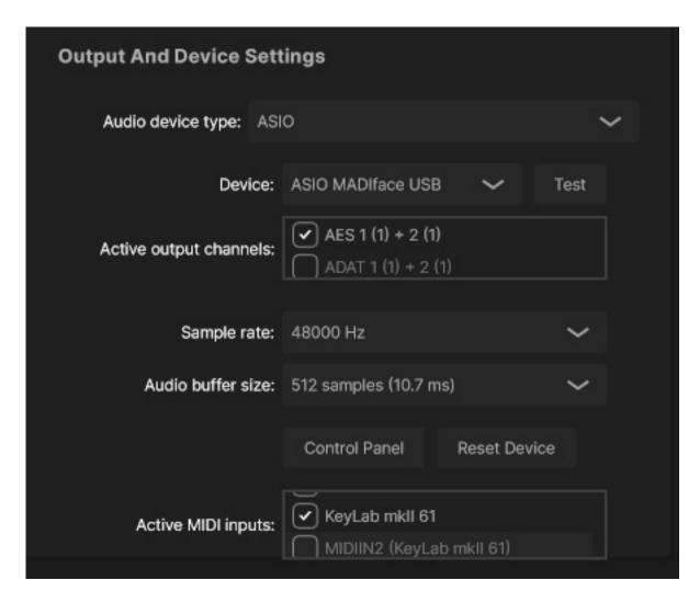
In the stand-alone version, an additional area appears where you can select the audio interface and the desired MIDI device. ASIO interfaces can also be used here.
