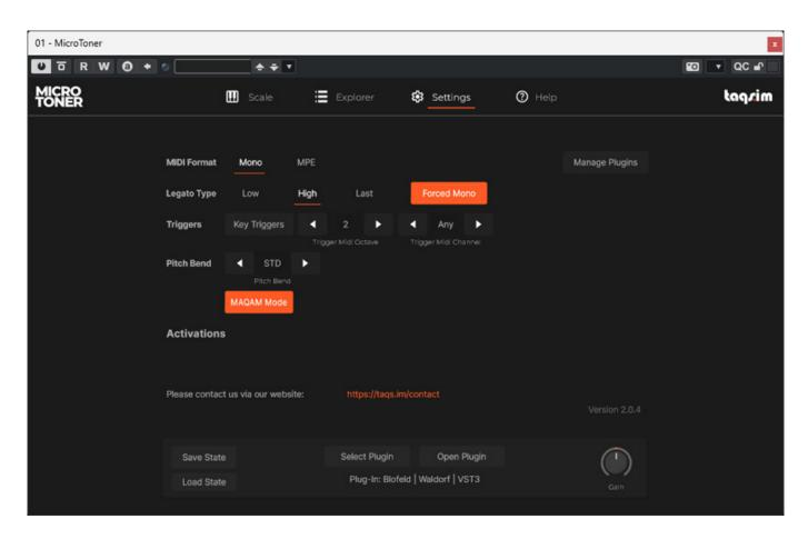
The MIDI parameters can be set on the "Settings" page. The pitch adjustment is done via MIDI pitch bend messages. By default, the pitch bend range is set to  $\pm$ - a semitone (STD). Of course, this must also be set accordingly on the synthesizer.
