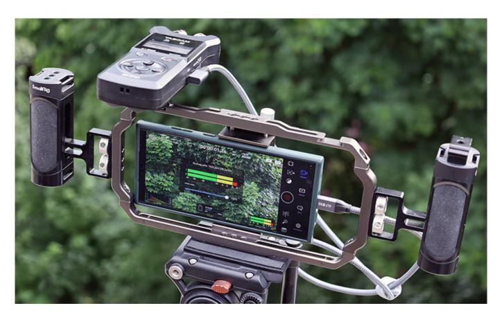
According to Tascam, support for Android systems cannot be guaranteed, unlike Apple iOS. However, the connection worked perfectly with the Samsung S23Ultra in our test. The DR-07XP was easily recognized as an external microphone in the DaVinci Resolve video app and worked without any dropouts in all recording sessions.
