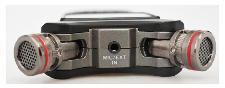
On the front panel, between the microphone capsules, there is a 3.5mm stereo jack input socket for external signals or stereo microphones.
