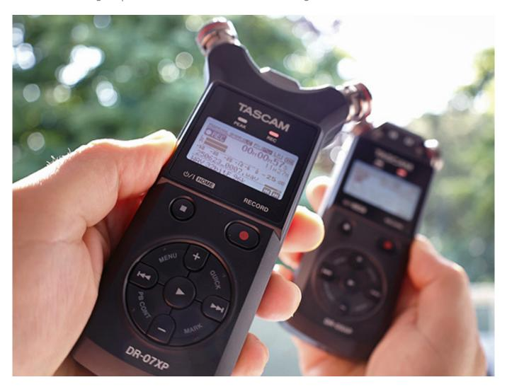
With the introduction of the latest generation of stereo audio recorders, Tascam has updated its already broad range of mobile recording devices. As successors to the acclaimed DR-05X and DR-07X recorders, the DR-05XP and DR-07XP now feature distortion-free recording using 32-bit float technology, and a sample rate of up to 96 kHz. In our test, we focus on the DR-07XP with foldable microphone capsules, as the two models differ primarily in their microphone technology.
