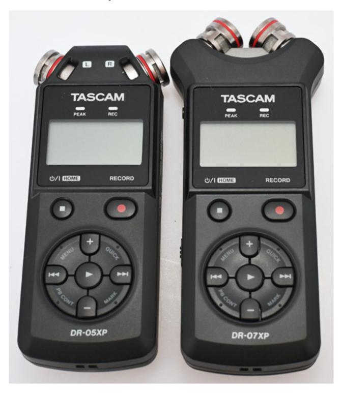
Both devices have identical connections and controls. A detailed, multilingual manual is included. The recorders feature a high-contrast, backlit monochrome display with a screen diagonal of 45mm and a resolution of 128 x 64 pixels,
