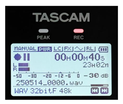
The backlit display is readable even in sunlight, and the buttons have a clear pressure point. When setting markers during the recording, the button sounds were audible due to the microphone capsules not being decoupled from the housing, as were other touches of the housing. This made it quite difficult to hold the device during an interview without picking up noise. A table or boom stand is recommended here.
