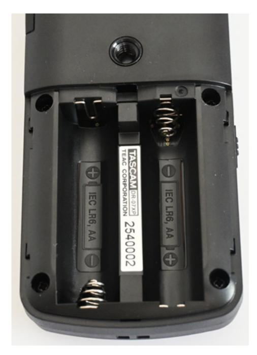
On the back, there is a 1/4-inch plastic tripod socket, a mono speaker with 0.3 watts of power, and a battery compartment for two alkaline batteries or NiMH rechargeable batteries (type AA).
