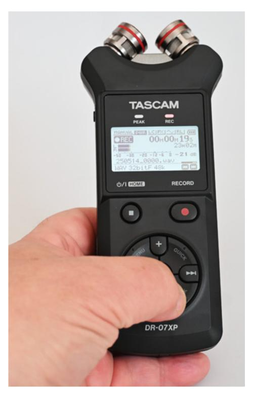
As with its predecessor and other multitrack devices in the Tascam family, the operation is well thought out and easy to understand without having to study the user manual, which can be downloaded online in English. Thanks to the well-structured menu navigation and button layout, the DR-07XP can be operated easily with one hand. I found the quick button very helpful, as it allowed me to edit important parameters directly in context, depending on the menu.
