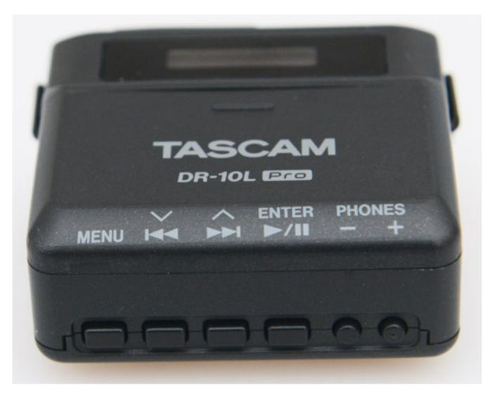
Pressing the MENU button opens the menu, which has 28 entries. Here, you can configure many settings on the device. Use the buttons |<< and >>| to select the desired menu option and confirm with the ENTER button. You can now change the parameter using the two buttons |<< and >>| and confirm with ENTER. This takes you back to the menu/parameter selection.
