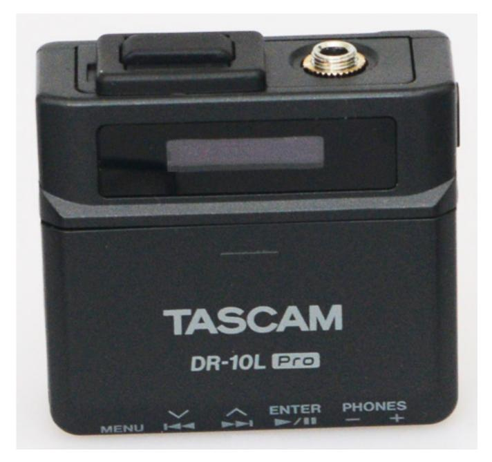
Let's take a look at a few more technical details. The maximum input level is -11 dBV and the connection impedance is  $>2k\Omega$ . The adjustable input gain ranges from 7.5 to 38dB. The frequency range is specified as 20Hz to 20kHz (0/-1 dB). The manufacturer specifies a dynamic range of 105dB or more.
