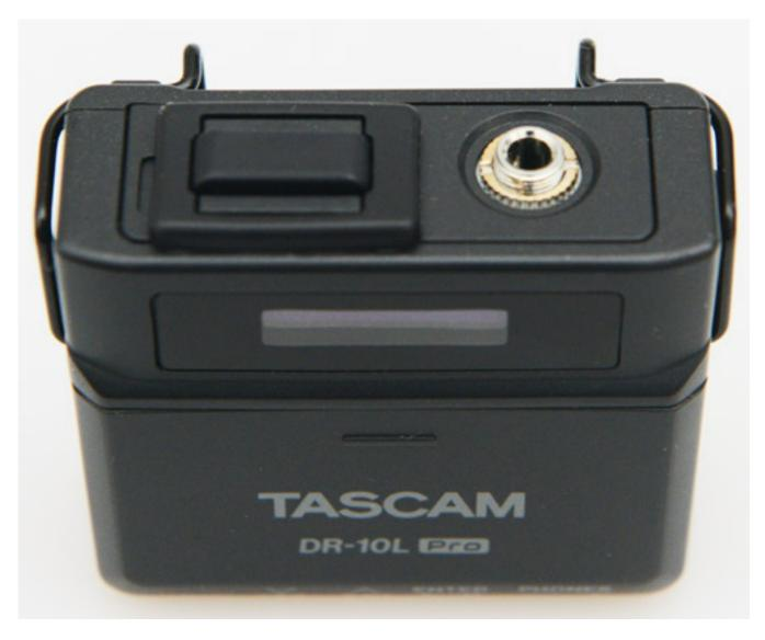
At the top is a 3.5mm TRS jack socket for connecting Sennheiser-compatible microphones. These can also be locked in place with the standard Sennheiser cap on the jack plug. The socket has a 2.3 volt bias voltage for the microphone.
