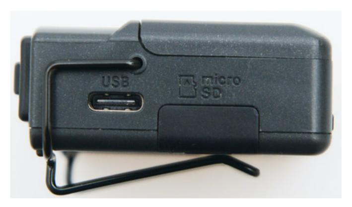
The USB interface is designed as a USB-C socket. Next to it is the cover for the SD card slot. MicroSD, MicroSDHC, and MicroSDXC cards (up to 512 GB) can be used for recording. The card can also be read with a connected computer in mass storage mode using the USB port. This mode can be activated via the menu on the DR-10L Pro.
