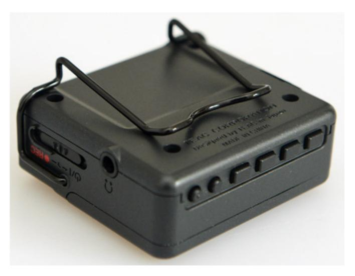
There is also a headphone output (see figure above) in the form of a 3.5mm TRS plug on the side. The maximum output is specified here as ten milliwatts per channel.
