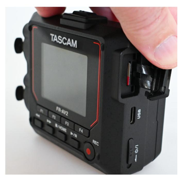
The USB 2.0 port is located on the right side. Incidentally, this not only enables twochannel output but also digital audio input via USB with sample rates of 48 and 96 kH, as well as word lengths of 24 bits or 32-bit float. The on/off switch for the recorder is located at the bottom, and the micro SD card slot is located behind a rubber cover.
