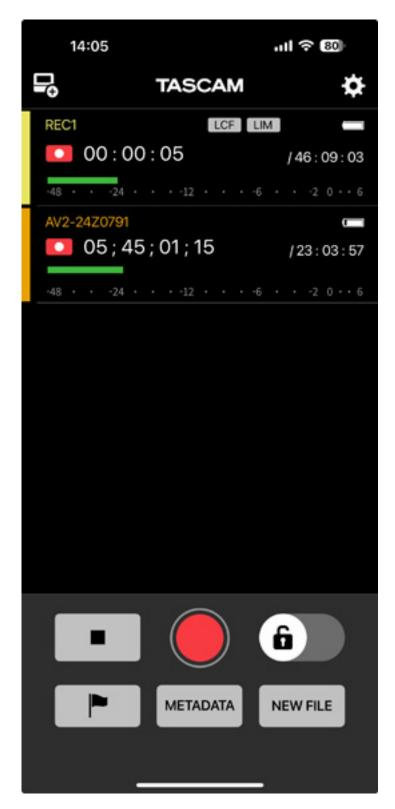
The record button at the bottom allows you to start recording on all connected devices simultaneously. In the app, it appears as if the recording starts at different times on the devices, but the start is completely synchronized.
