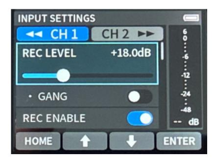
The INPUT dialog allows you to adjust the recording level and link the channels (GANG), select the input or source (mic, line, external, or USB), select stereo/mono, and activate phantom power for each channel individually.
