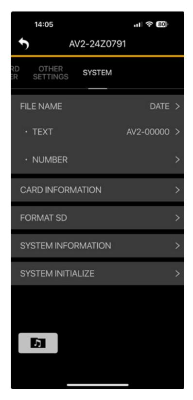
The SYSTEM page allows you to configure the file name format, format the SD card, and view system information.
