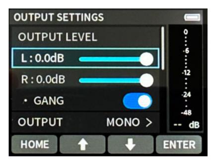
The OUTPUT dialog also allows you to set the level and link the level settings, select the level range (line/camera), switch between mono and stereo, and add a limiter and delay.
