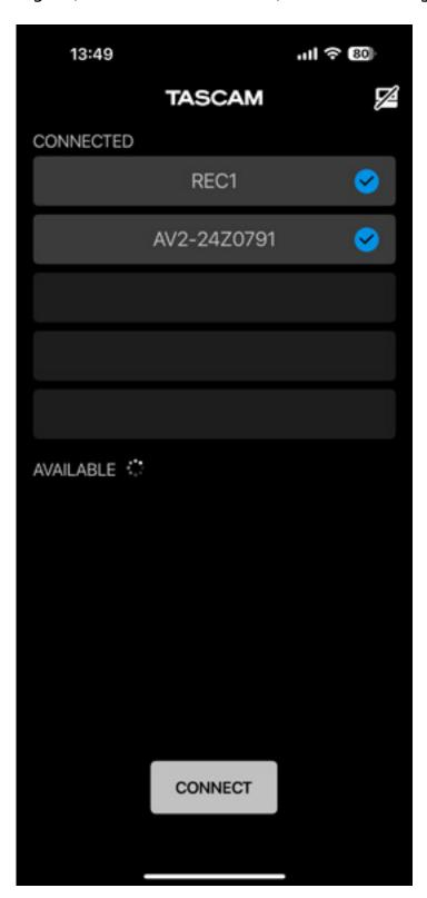
Multiple compatible devices can be connected simultaneously. Here, in our example (see fig. above), an FR-AV2 and a DR-10L Pro are connected. The connection is established directly through the app, and you don't have to go into the Bluetooth configuration of your smartphone or tablet operating system.
