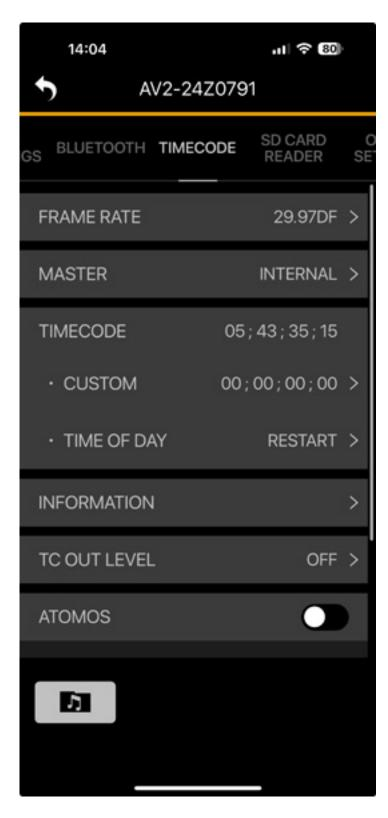
For Bluetooth, the audio monitoring quality can be set to three levels (Prime, Standard, Stable). In addition to the usual parameters in the timecode menu, you can also activate synchronization with Atomos products via Bluetooth and establish or disconnect a connection to an Atomos device.
