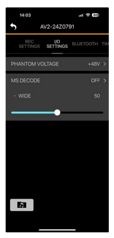
In the I/O settings, you can switch the phantom power, activate the MS decoder, and set the stereo width.
