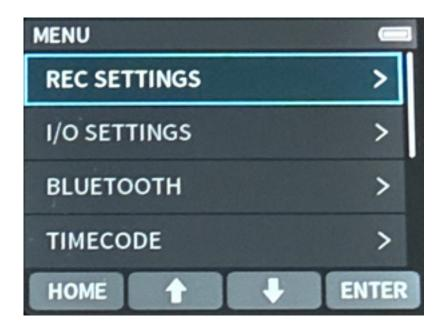
The global menu contains dialog pages for setting the recording parameters (sample rate 48, 96 or 192 kHz, word length, pre-recording, etc.), for the inputs and outputs, for Bluetooth, timecode, system-related items, and a dialog for miscellaneous items. Here, you can also activate an auto slate tone and adjust the slate tone level.
