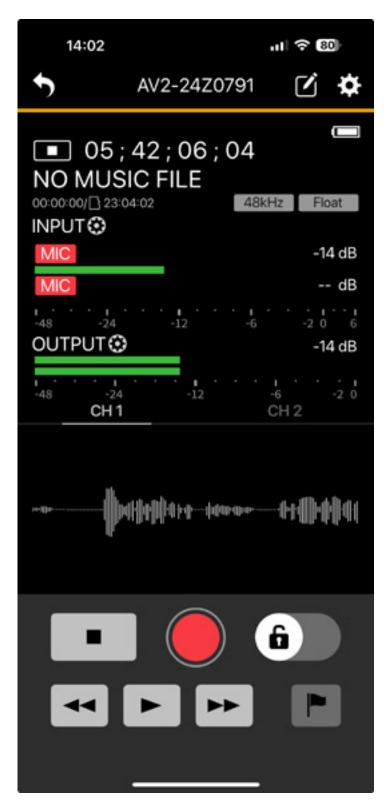
Here (see image above) is a view of the overview screen of the FR-AV2 selected in the app, along with a meter and amplitude curve.
