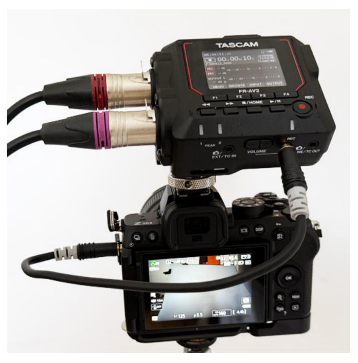
In continuous recording mode with phantom power and 32-bit float/48kHz, normal alkaline batteries last for approx. 4 1/2 hours and without phantom power even twice as long. When using lithium batteries, the runtime in continuous operation increases by more than double.
