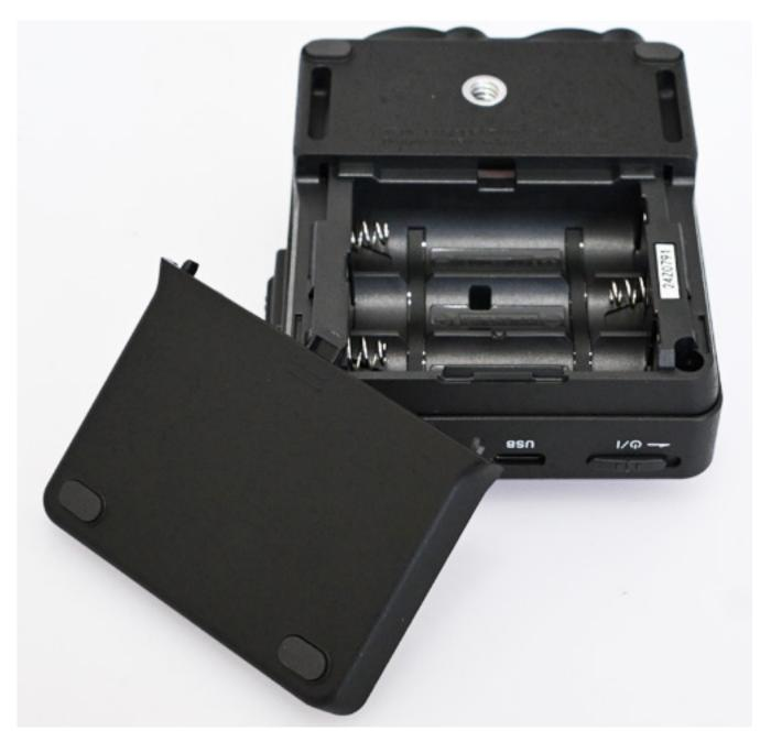
The recorder is powered by three AA batteries (alkaline, NiMH rechargeable, or lithium can be used), which can be inserted after removing the cover. It can also be powered via USB, and an external power supply is available as an option (PS-P520U).
