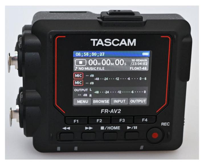
Now let's take a look at the controls on the front of the device. There is a 42  $\times$  30mm color display. Below that, four function keys can be found, whose current function is shown on the display. There are also four transport keys for pause/play, stop, and fast forward/rewind, as well as a key for starting recording. Recording is stopped with the stop/home button.
