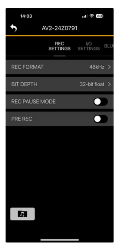
Clicking on the gear icon opens the configuration menu with various dialogs. Here, you will first find the parameters for recording, such as sample rate, word width, record pause mode, and pre-recording function.
