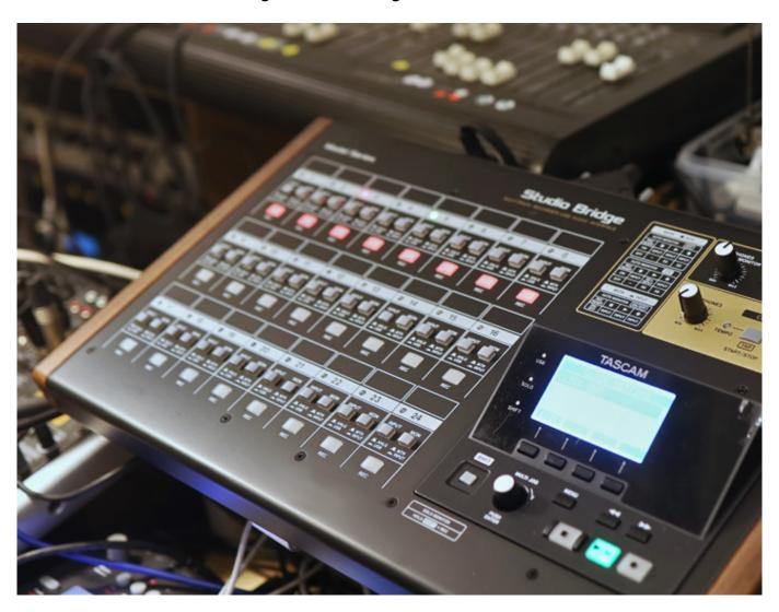
Studio Bridge is in the format of a desktop device. With a separately purchased kit, Studio Bridge can also be mounted in 19-inch racks. To do this, you have to remove the visually appealing side panels with a wooden finish. On a table or stand, the Studio Bridge stands at a slight angle. With dimensions of  $446.5 \times 114.6 \times 269.5$  mm, it weighs 4.5 kg.
