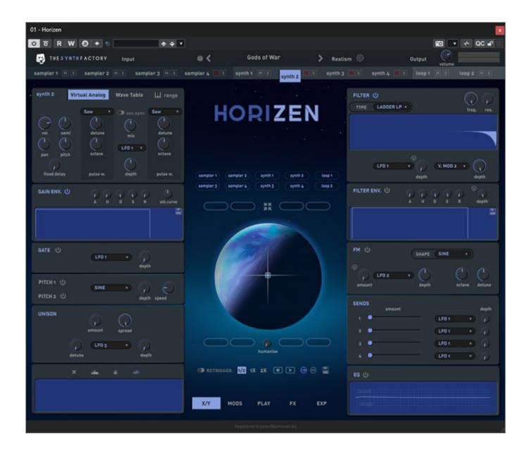
The concept of Horizen is based on up to ten parallel voices: four voices with samples, four synthesizer voices, each with two oscillators with fixed waveforms or wavetables, and two loop players. This guarantees complex sounds.
