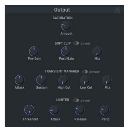
And on the far right, there is a button for calling up the output dialog, where you will also find a saturation effect with adjustable intensity, as well as switchable soft clippers, a transient manager, and a limiter (see image above). That concludes our brief overview of Horizen's features.
