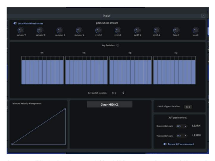
At the top of the header, there are additional dialogs that can be opened. To the left of the preset selection, there is an input dialog for keyboard velocity, keyboard range assignment, MIDI CC, and parameter assignment to the X/Y pad.
