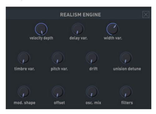
The "Realism Engine" allows the user to simulate analog tolerances for various
