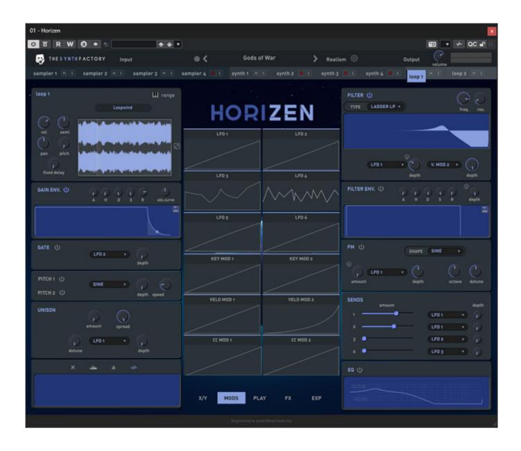
In the Modulation tab, in addition to six LFOs, there are two modulation options each for keyboard tracking, velocity, and MIDI CC (see image above).
