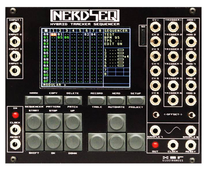
At this point, let's consider a look at the buttons for operating the NerdSEQ. The upper row of buttons with smaller buttons is used to call up individual pages or dialogs, such as Sequencer, Pattern, Patch, Table, Automate, and Project. In conjunction with the Shift key, you can call up additional functions using these keys, such as mark, copy, delete, start recording, settings, etc.
