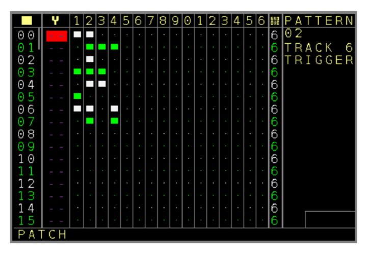
For tracks with assigned trigger-out expanders, there is also a page on which the user can view a grid display to set triggers for individual outputs per step (see illustration above). This editor page is somewhat hidden and you have to scroll through to find the end.
