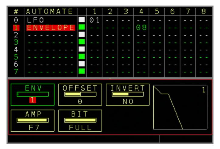
You can also modulate signals using the existing LFOs and envelopes. The modulation matrix for this can also be selected via the AUTOMATE menu (see illustration above). This allows the realization of very complex processes.
