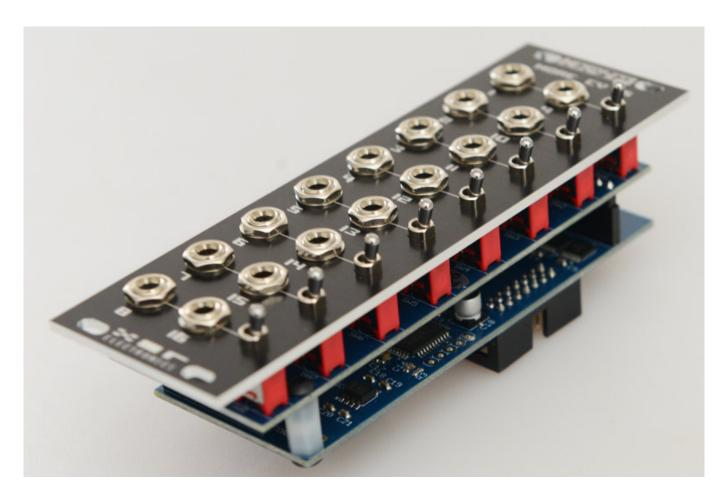
The CV16 expander has 16 CV outputs (3.5 mm jack sockets). One pair each (1/9,  $2/10 \dots 8/16$ ) can be selected in the voltage range of -5 ... +5 or 0 ... +10 volts via a miniature toggle switch.
