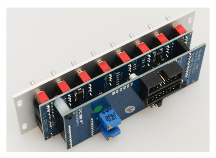
The module is not merely a D/A converter; it is also equipped with a microcontroller. It also supports the output of LFOs or envelopes. But more on this later. The price of the 16CV expander is less than 160 euros. The module is available in three versions: gray, black, and gray/black (black with gray edge).
