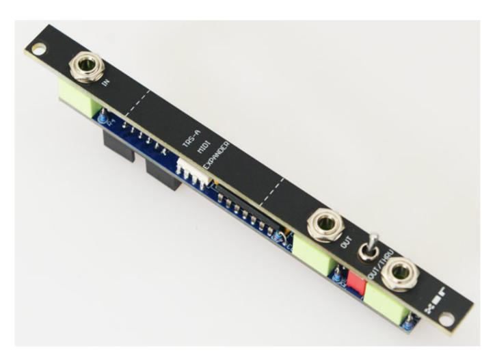
Let's start with the hardware options. As an alternative to the I/O expander with MIDI interface (inputs and outputs designed as 5-pin DIN sockets), the new MIDI interface with a width of just 2 HP offers a MIDI In and a MIDI Out as well as an additional switchable output that can be used as a MIDI Thru or second MIDI Out via a mini toggle switch.
