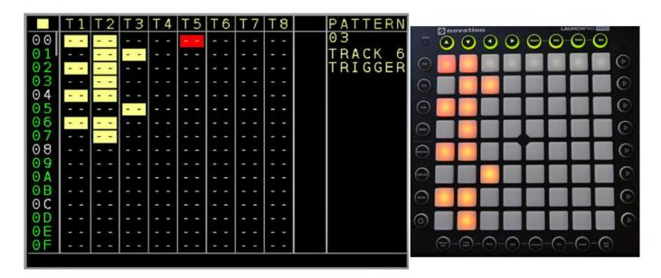
When a pattern is opened, the corresponding entries are also displayed. This is particularly useful for patterns whose track are assigned to a MORE TRIGGERS 16 module (see illustration above). Here, you can program drums/percussion very easily and quickly using the launchpad via the drum matrix page.
