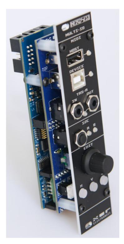
In addition to the I/O expander with DIN jacks and a connection for the Sega Gamepad, as well as the compact 2HP MIDI expander with mini TRS jacks, there has been a third expander with MIDI since 2024: the multi-IO expander. This expander with a width of 6U not only has MIDI but also offers additional functionality, such as an I2C connection and an encoder with three function keys.
