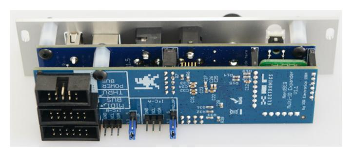
On the back, there are three connectors for the power supply and the internal MIDI bus, as well as a MIDI-Thru to which you can connect another gamepad expander. The connector is not intended for further MIDI expanders because in a NerdSEQ system, MIDI is only supported by one expander.
