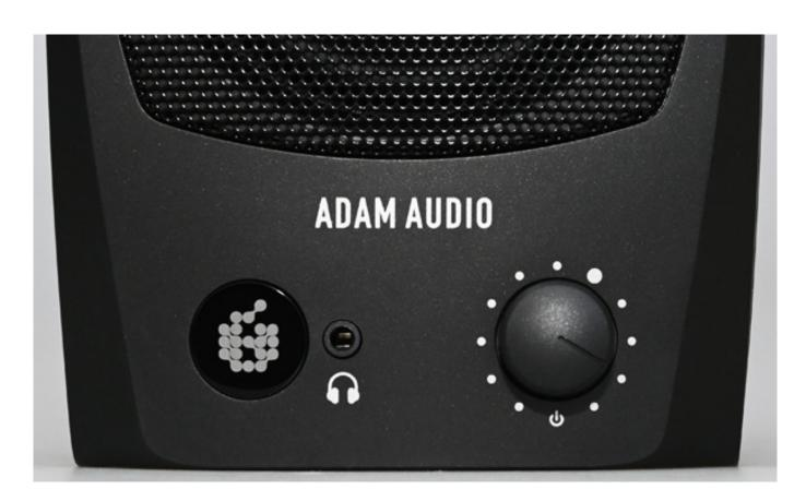
On the front of the left speaker, there is a 3.5mm jack socket (TRS) for connecting headphones (output impedance 32 ohms) and the volume control, which also offers a push-button function that can be used to turn the system on and off, select the signal source (analog or USB), mute the speakers and swap channels. The status is indicated by the color of the display next to the headphone output. Cyan means USB connection active, green means analog inputs and yellow flashing means mute, for example.
