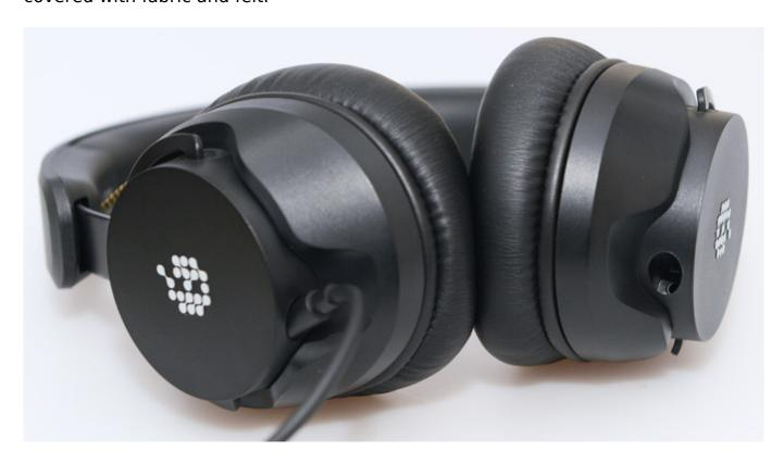
The weight of the headphones is about 250 grams without the cable, and the housing is made of 85 percent recycled ABS plastic. A 2.5-mm jack socket is provided on both sides of the headphones for connecting the headphone cable. The cable can therefore be plugged in on the left or right (see figure above) and is mechanically locked to prevent accidental unplugging.
