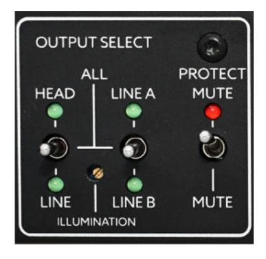
The output section features two three-way switches for line/headphones and line A/B. In the center position, both functions are active. There is also a switch for mute and a status LED in case a protective circuit is activated. Incidentally, there is a delay before the headphones are switched on, and the MC50 also features a temperature monitor to protect the device.
