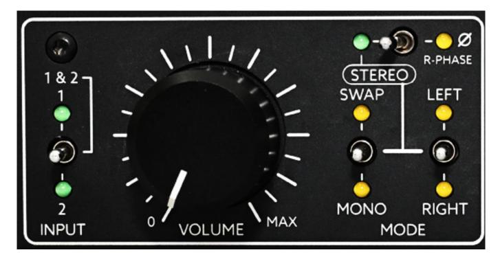
In the input and monitor section (see figure above), one of the two inputs can be activated, and in the center position, both can be activated simultaneously. A high-quality RK27 potentiometer from Alps, with 41 clicks, is used for the input level (knob diameter 25 mm). To the right of the volume control, there are three switches for the monitor functions, such as: phase reversal, channel swap, or mono, as well as the selection of only the left or right channel, or both.
