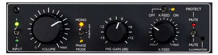
The controls on the Lake People G114 are limited to input selection, level adjustment, mono/phase reversal, pre-gain adjustment, crossfeed, and mute.
