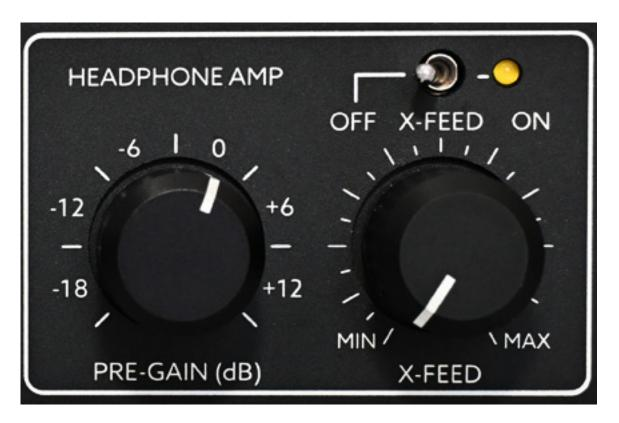
On the MC50, a pre-gain can also be set in the headphone section, ranging from -18 to +12 dB, so that at nominal monitoring volume, the level control is approximately in the middle of the control range. This means that you don't have to fiddle with the DIP switch inside the device and can quickly make adjustments if you want to use headphones with different impedances or sensitivity. The headphone section also offers a switchable and then adjustable crossfeed (X-FEED).
