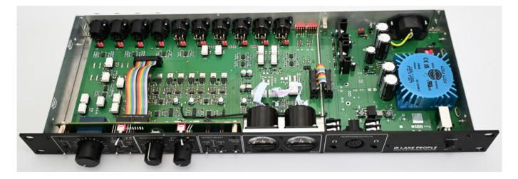
In February 2025, we already had the opportunity to test a pre-production model, which, however, was technically the same as the production model. The housing (483 x 44 x 188 mm) is made of stainless steel, and the front panel is made of three-millimeter aluminum. The integrated power supply (115/230 V, switchable
