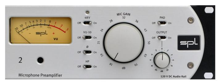
The SPL Crescendo Duo offers two input channels with up to 70dB of gain and two outputs per channel, the gain of which can be boosted by 10dB using the "Output"-switch independently of the input gain. This allows the user to feed optimal signal level to components further down the chain. The large rotary knob is detented, internally raising the gain by increasing amounts from +1 over +4 up to +7dB. The rotary control for output gain is stepless.
