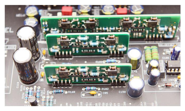
The two smaller boards mounted consecutively are the two SUPRA opamps. A larger board right behind houses the elaborately confectioned circuit responsible for electrically balancing the symmetrical signal.
