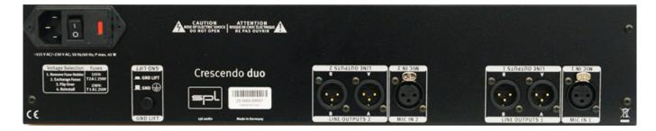
The rear of the enclosure sports an IEC socket, on/off-switch, one XLR input per channel plus two parallel line-level XLR outputs. Very useful for backup purposes. Input impedance is rated at ten kiloohm and output-impedance at 75 ohm. The maximal output level goes up to 32.5dBu. The phantom-power circuit suplies a whopping 35mA per channel, satisfying even the most picky contenders.
